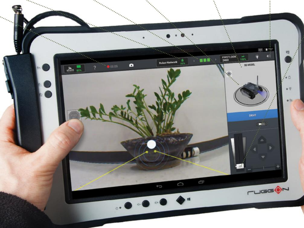
The image shows a person's hands holding a ruggedized tablet controller. The screen displays a live video feed of a potted plant with a robot's camera view overlaid. On the right side of the screen, there is a 3D model of the robot and a control panel with a "DRIVE" button and directional controls. The top of the screen shows a status bar with "Robot Network 85%", "FIRSTLOOK 2460 100%", and a battery icon. The "FLIGGEON" logo is visible at the bottom of the tablet.
